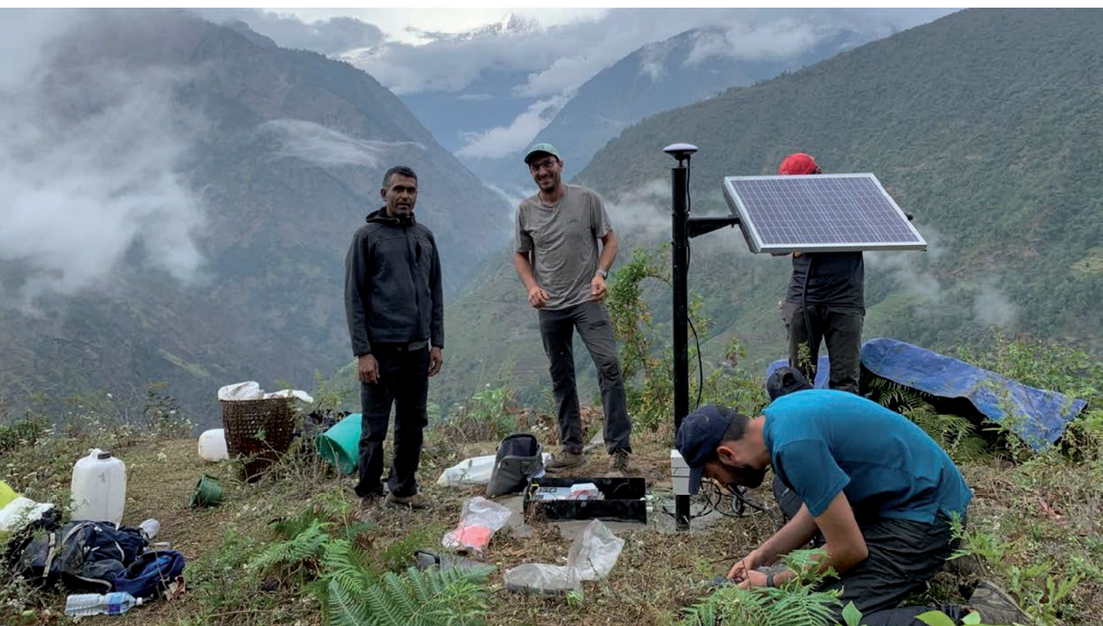
Installation of a GNSS and seismic station on the Bolde landslide, Central Nepal (Photo: M. Jaspard)
